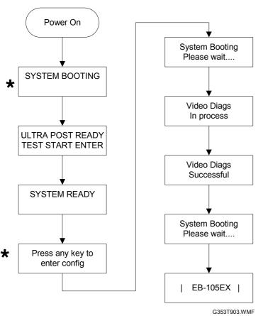
★ There is no need to press any key when you get this message during the normal booting sequence. After the EB-105EX becomes idle, press the Fiery Menu key and the Fiery menu screen (Fiery information screen) will appear on the copier operation panel.
