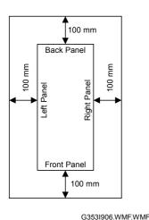
Place the machine near the power source, providing clearance as shown.
