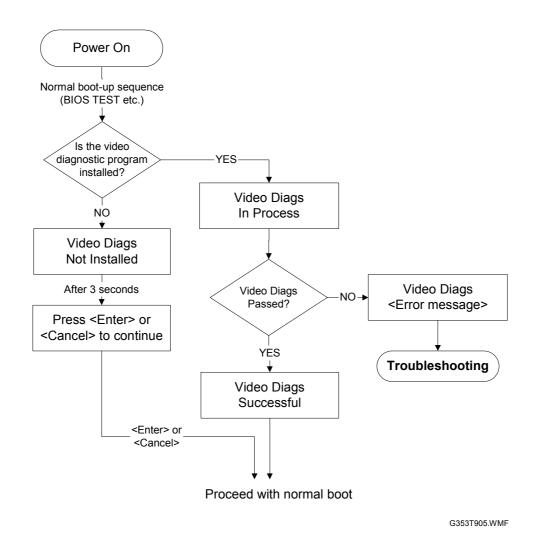
When video board diagnostics detected an error, an error message will appear on the LCD message panel, until you power off the EB-105EX and the problem has been solved.
